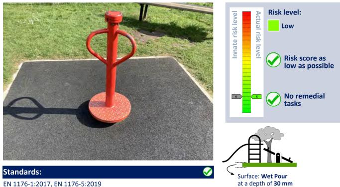
EN 1176-1:2017, EN 1176-5:2019 The item and its surfacing (where applicable) meet with the requirements of the relevant standards.
